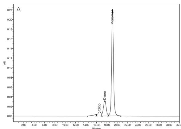
*Figure 1: Example HPLC chromatograms with peaks representing BSA in its oligomer, dimer, and monomer states. Chromatograms A and B have 77.1% and 94.2% BSA monomer, respectively.*
